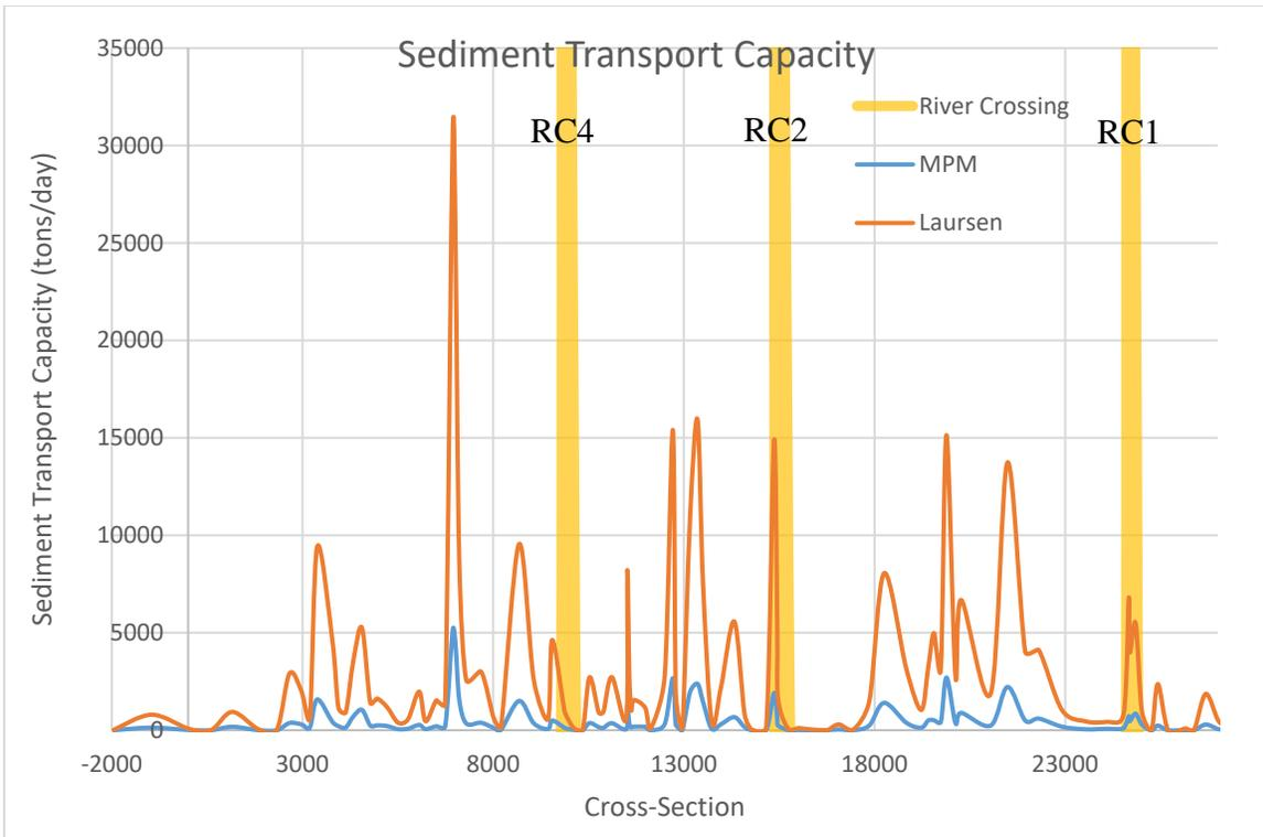
Figure 3.6 MPM and Laursen Sediment Transport Capacity for the system AS IS
