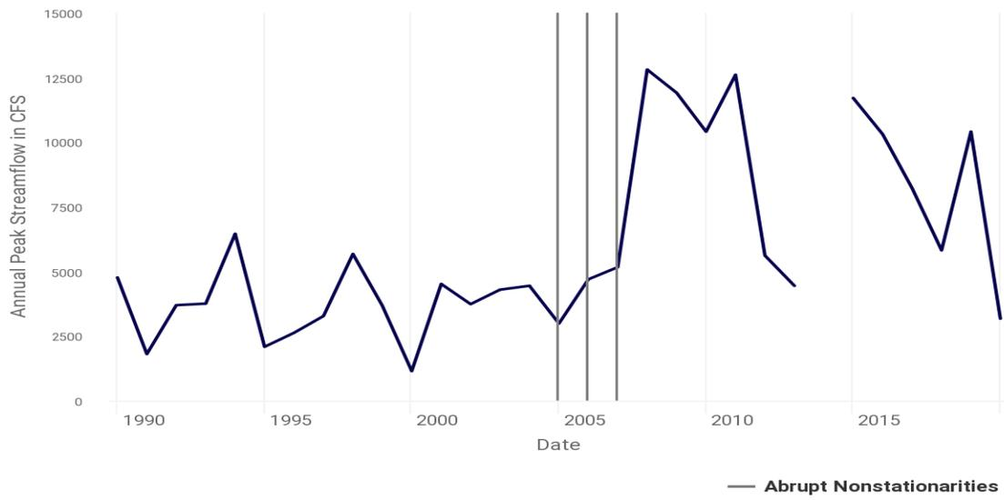
Figure 4.2 Abrupt Nonstationarities in Annual Peak Streamflow for Maumelle River at Williams Junction, AR
