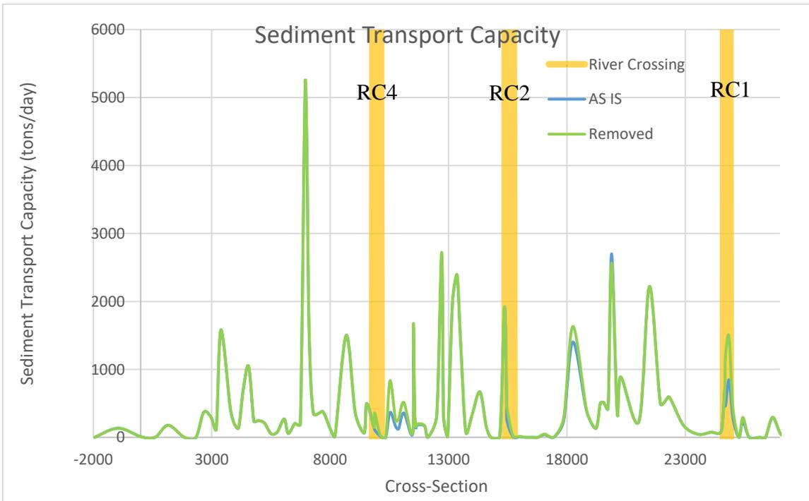
Figure 3.10 Sediment Transport Capacity for AS IS and after river crossing removal
