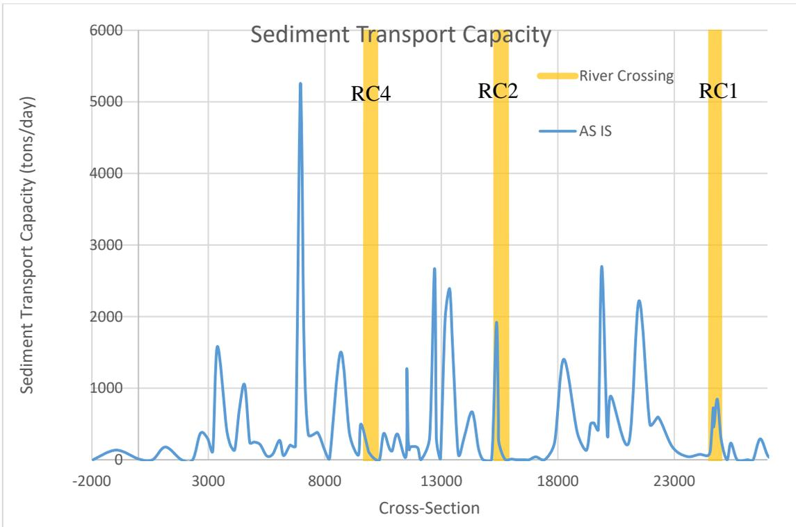
Figure 3.9 Sediment Transport Capacity for AS IS condition
