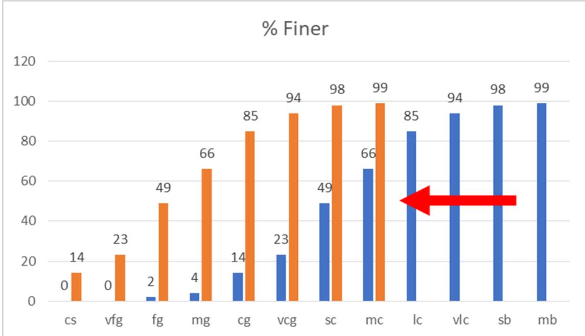
Figure 3.7 Shifted Grain Size Distribution for Sensitivity Analysis
