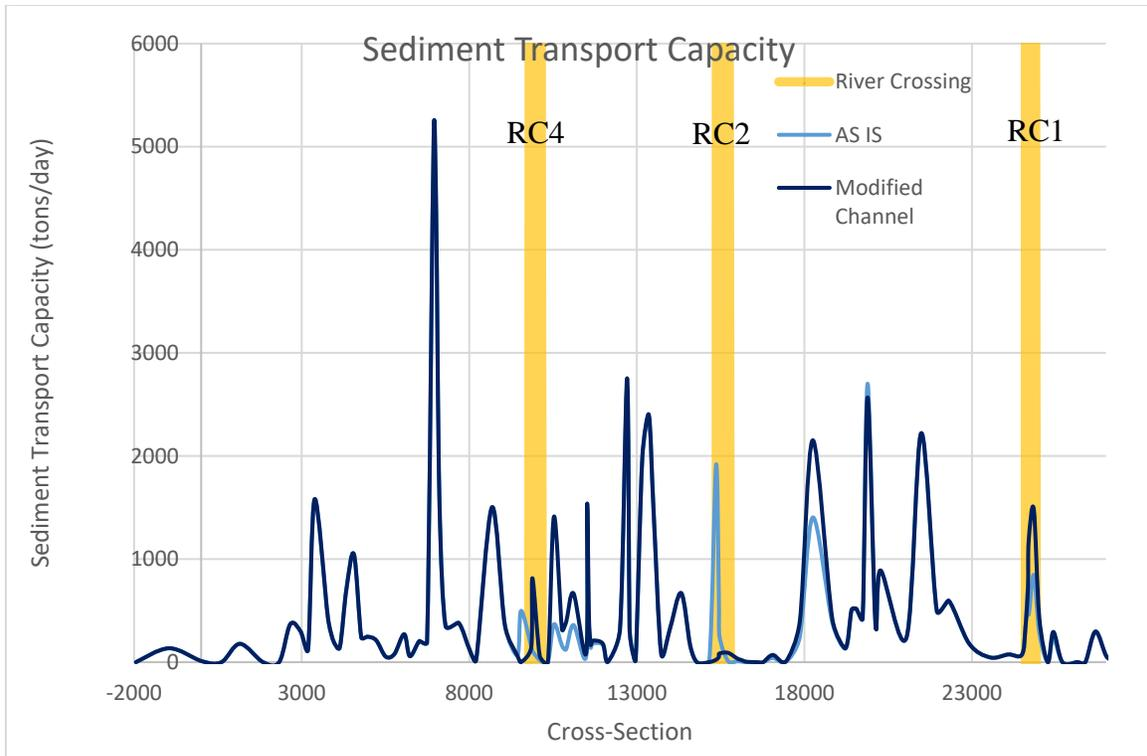
Figure 3.11 Sediment Transport Capacity After River Crossing Removal and Channel Modification
