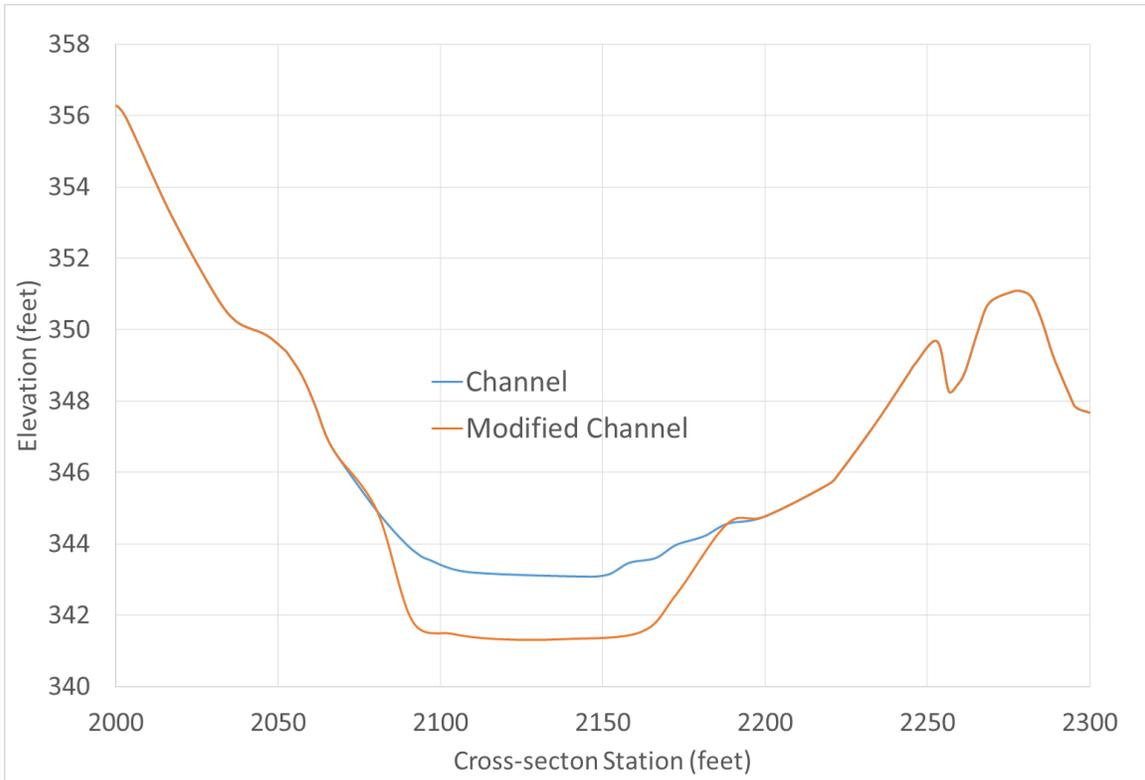
Figure 2.5 Channel in Removed Scenario and Modified Channel
