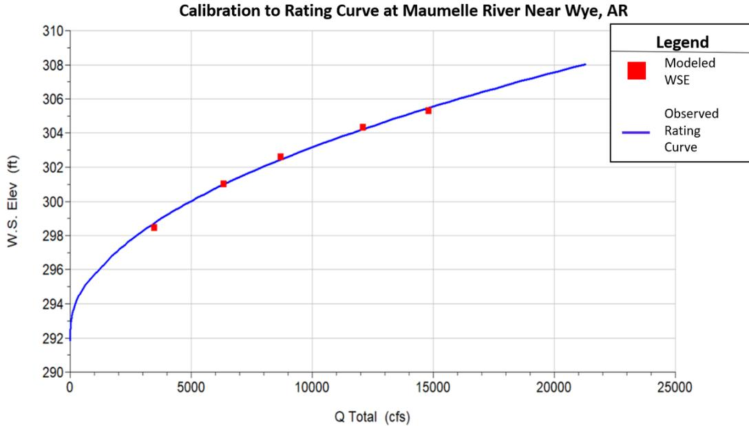
Figure 2.4 Calibration to Rating Curve at Maumelle River Near Wye, AR (07263296). Observed (blue) and Modeled (red) Rating Curve
